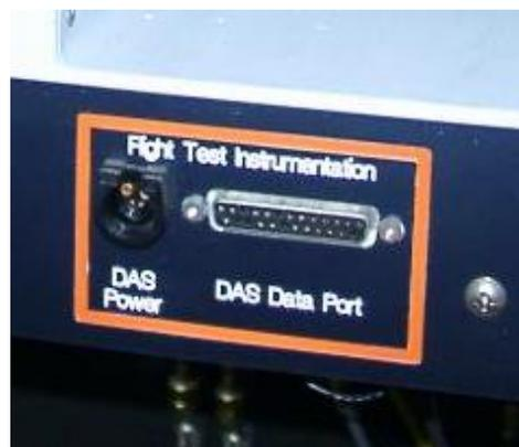
**ARINC 628 Socket Installed in Panel**
